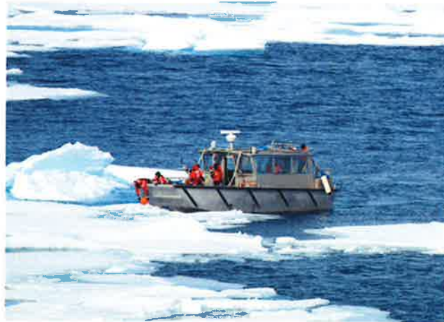
The crew of the icebreaker Healy lowering an iSphere onto an ice floe to simulate tracking oil in ice. (NOAA/Jill Bodnar)
