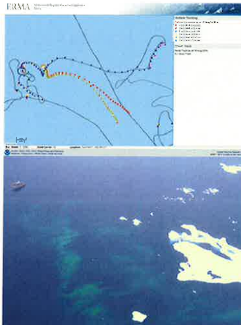
Above, Arctic ERMA displays iSphere positional updates. The blue and purple points remained on the Healy as a "control" against the ship track, while the red, orange, green & yellow tracked ice floes and followed surface currents. Below, taken from 300 feet in the sky, Puma
